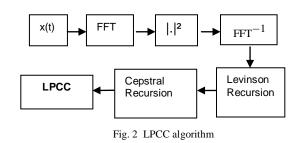
First, Fourier transform of the signal is applied. Then, calculating the inverse Fourier transform of its module squared. Finally, we pass to Levinson and cepstral recursion for getting LPCC coefficients.
