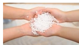
Fig. 1 Polystyrene granules, whose density is 35 kg / m 3
