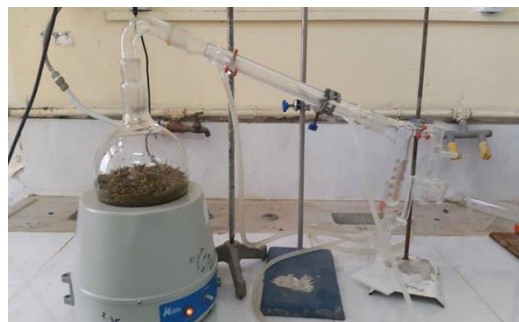
Figure 03: Installation of a modified clever type hydrodistillator, made at the ecology laboratory (UMBB).
