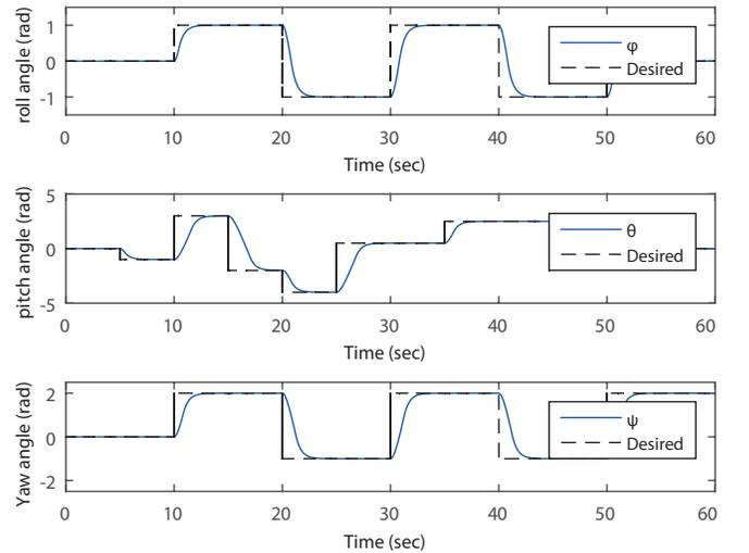
Fig. 2. SMC- based results for the attitude tracking of the Quadrotor.
