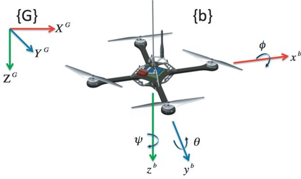
Fig. 1. Mechanical structure of the Quadrotor and related frames.
