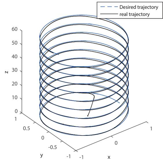
Fig. 6. SMC- based helical path tracking of the Quadrotor.
