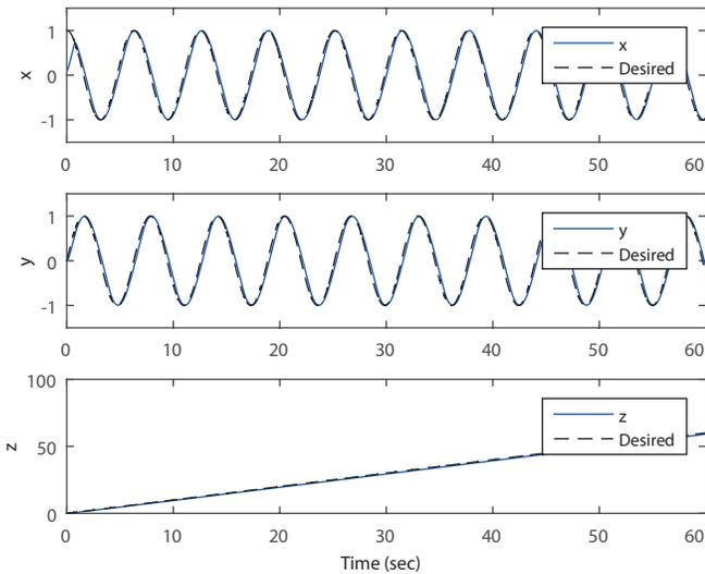
Fig. 4. SMC based results for the position tracking of the Quadrotor.
