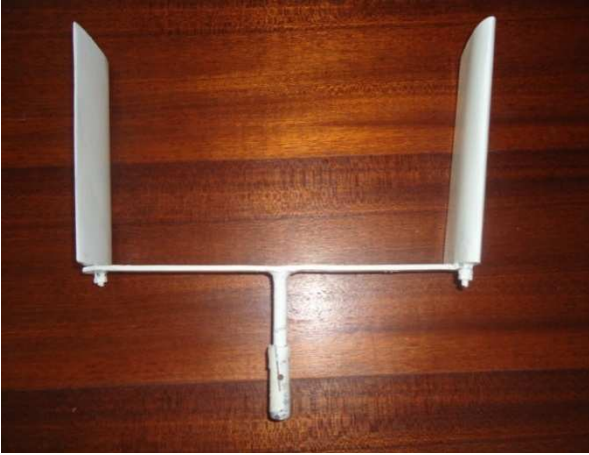
(a) Darrieus rotor (for measurement of C_L and C_D )
