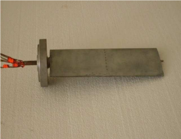
(b) Blade with NACA0015 profile (for pressure measurement)
