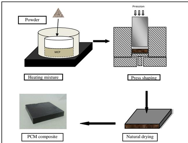
Figure1. Preparation schematic for the thermal storage materials
