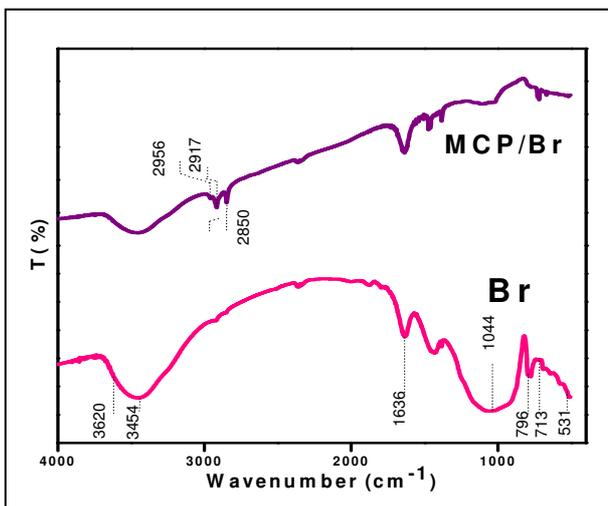
Figure3. FT-IR spectra of the red brick powder and the PCM/Br composite
