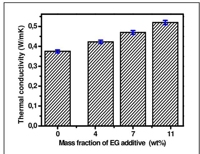
Figure5. Thermal conductivity of PCM/Br composite containing EG
