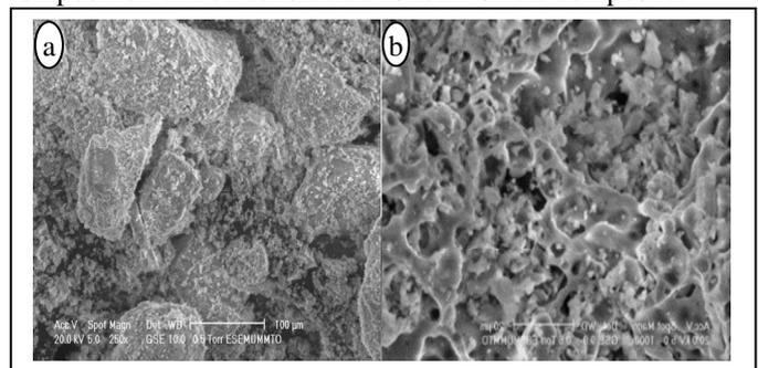
Figure2. ESEM photograph of the red brick powder and the PCM/Br composite
