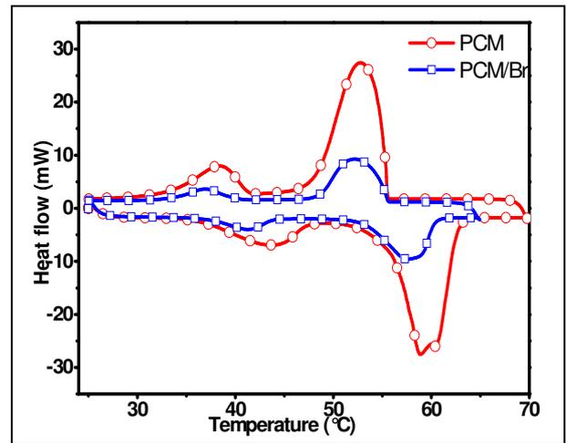
Figure4. DSC curves of PCM and PCM/Br composite.
