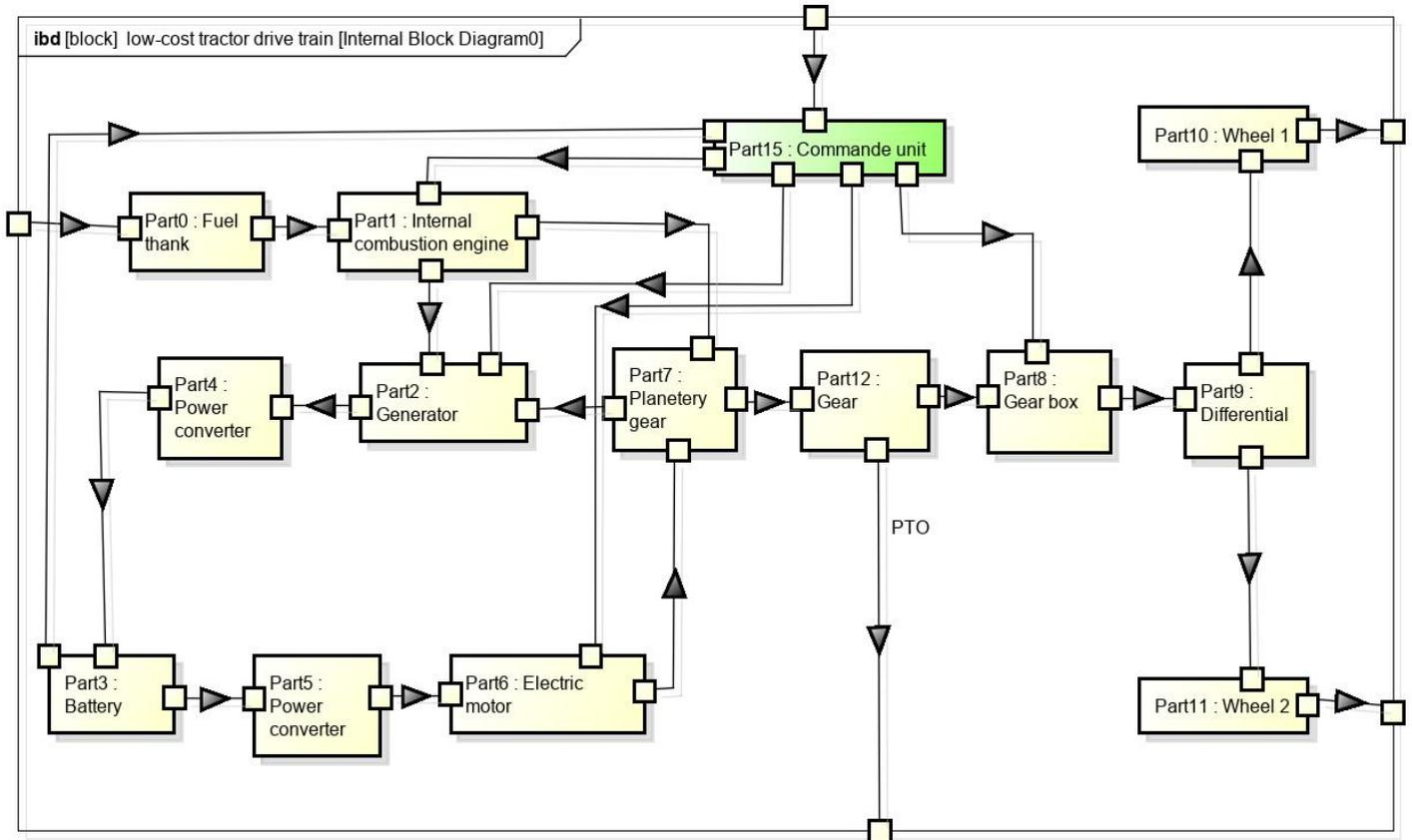
Fig. 4 Internal block diagram of the drive train of the low-cost tractor.
