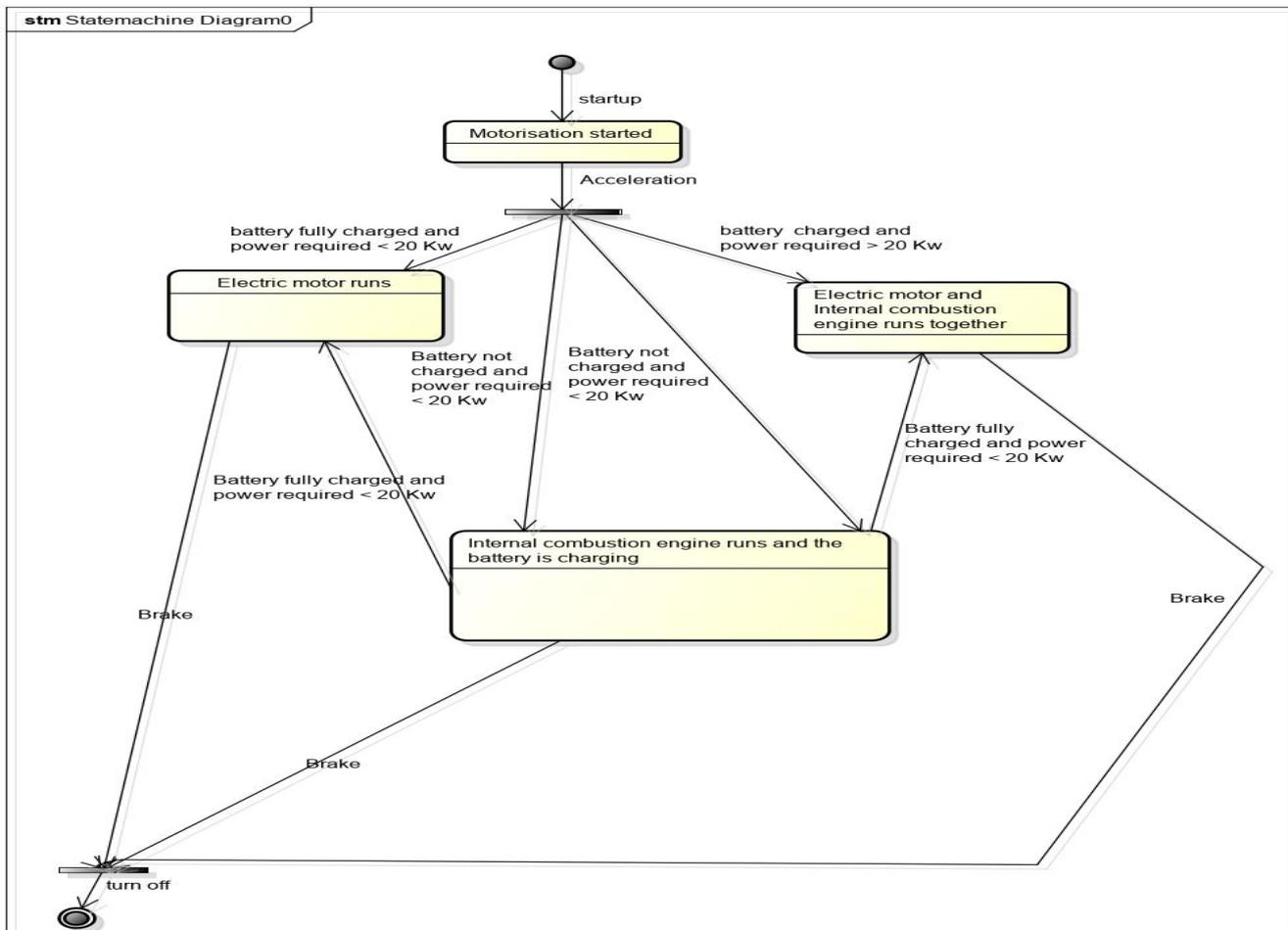
Fig. 5 StateMachin Diagram of the drive train of the low-cost tractor.
