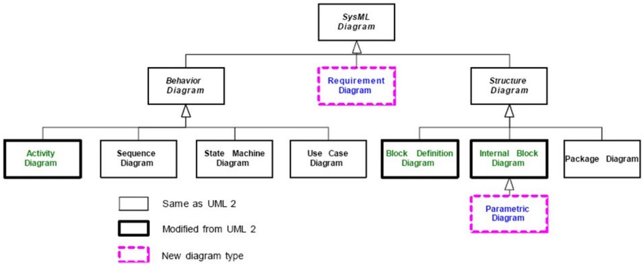
Fig.1 The nine diagrams according to the four pillars of modeling in the SysML language
