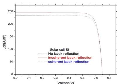
Fig. 3 show the characteristic the curve of  $J = f(V)$  for solar cell based on Si.
