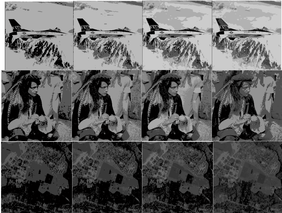
Figure 2. Results of segmentation with 2, 3, 4, 5 thresholds, respectively from (left to right)
