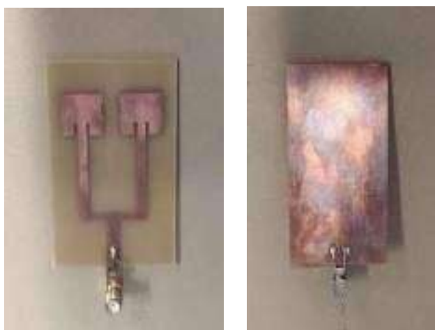
Fig.24. Antenna array (2×1) to be made (upper and lower face).
