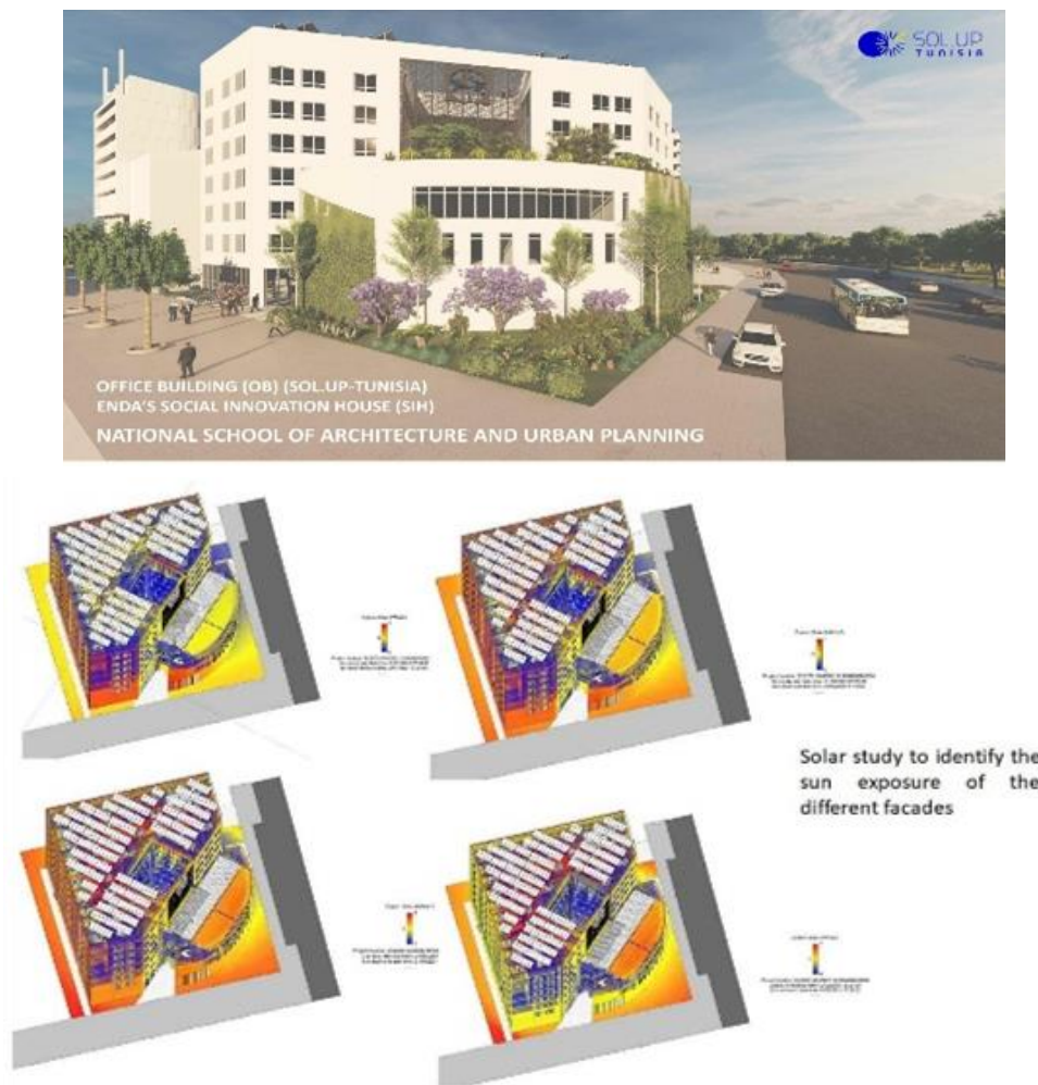
Fig 17: Office Building Project 2021. Perspective and Solar analysis
