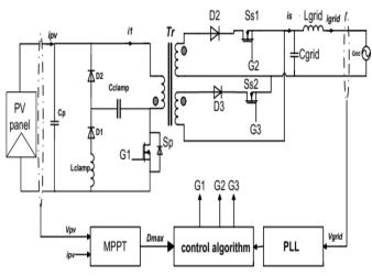
Fig.1. Flyback micro inverter and LCDD snubber
