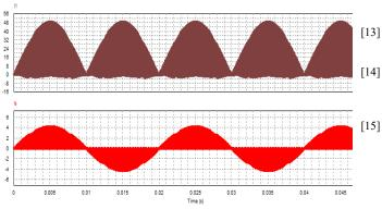
Fig.6. Primary current i1 and Secondary current is
