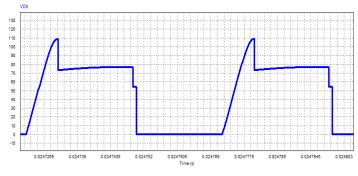
Fig. 5. Stress Drain Source voltage Sp switch
