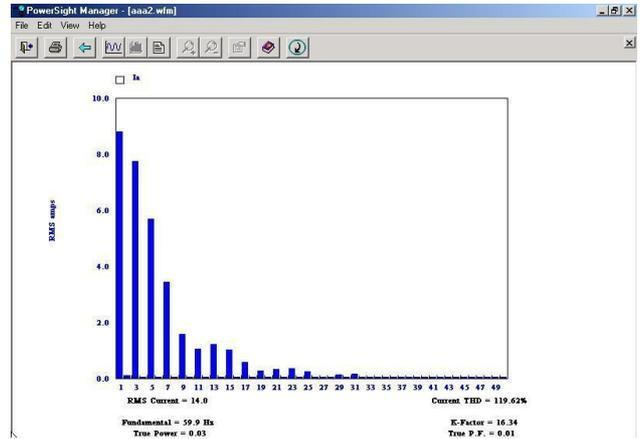
Fig. 10 Spectral Analysis showing the fundamental and the harmonics
