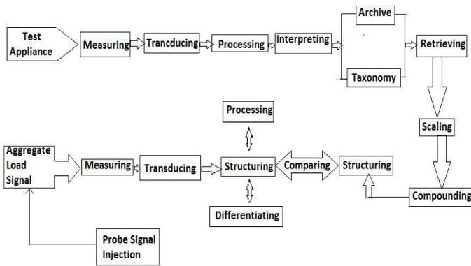
Fig. 2 Identification process of a load [1]
