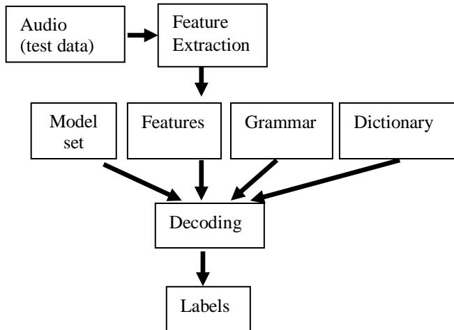
Fig. 6 Recognition schema
