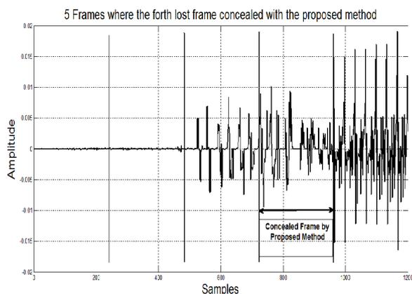
Fig.4 Concealed frame excitation by the proposed PLC method.
