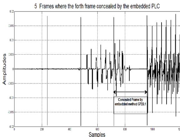
Fig.3 Concealed frame excitation by embedded G723.1PLC method.
