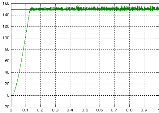
Fig. 11 Speed of the asynchronous machine with the application of the fuzzy control
