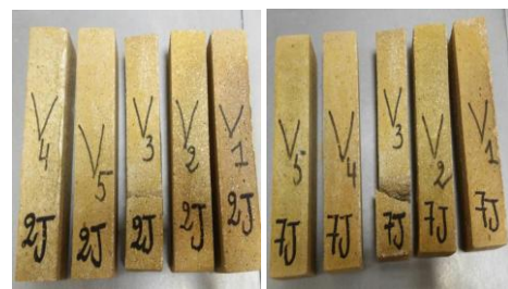
Fig. 5 Test specimens after heat treatment at 1400°C.
