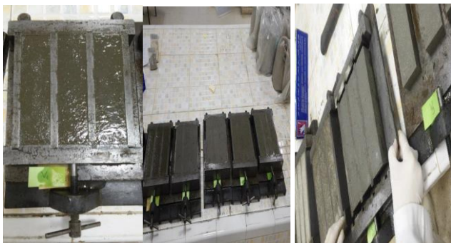
Fig. 1 Manufacture of mortar specimens
