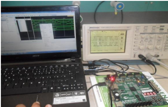
Fig.8 Photograph of the DSO display the control signals based on NR and generated from FPAG- XILINX
